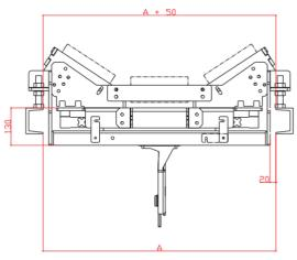
A-internal distance of the conveyor frame 600....1500mm
